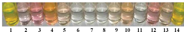
Fig. 7 (1) Dye 3 , (2) receptor 2 + dye 3 (1 : 1) = B . B with 1 equiv. amount of (3) \text{Cl}^- , (4) pimelate, (5) succinate, (6) \text{H}_2\text{PO}_4^- , (7) tartarate, (8) malate, (9) adipate, (10) N -Ts glutamate, (11) malonate, (12) acetate, (13) glutarate, (14) citrate; [\mathbf{3}] = 8.5 \times 10^{-5} \text{ M} , [\mathbf{2}] = 4.2 \times 10^{-4} \text{ M} , [\text{G}] = 2.0 \times 10^{-3} \text{ M} in \text{CH}_3\text{CN}-\text{H}_2\text{O} (4 : 1 v/v, 10 mM Tris HCl buffer, pH = 6.3).
